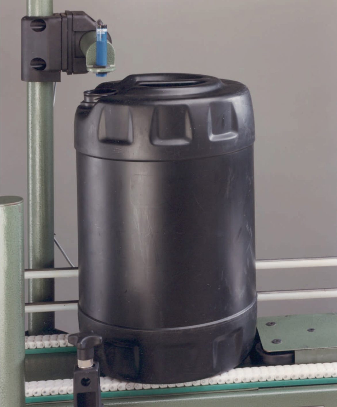
Turning device for aligning round containers, Sensor detects bung opening.
